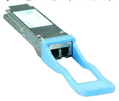
Figure 8-12 Appearance of a QSFP28 optical module (for LC optical fibers)
