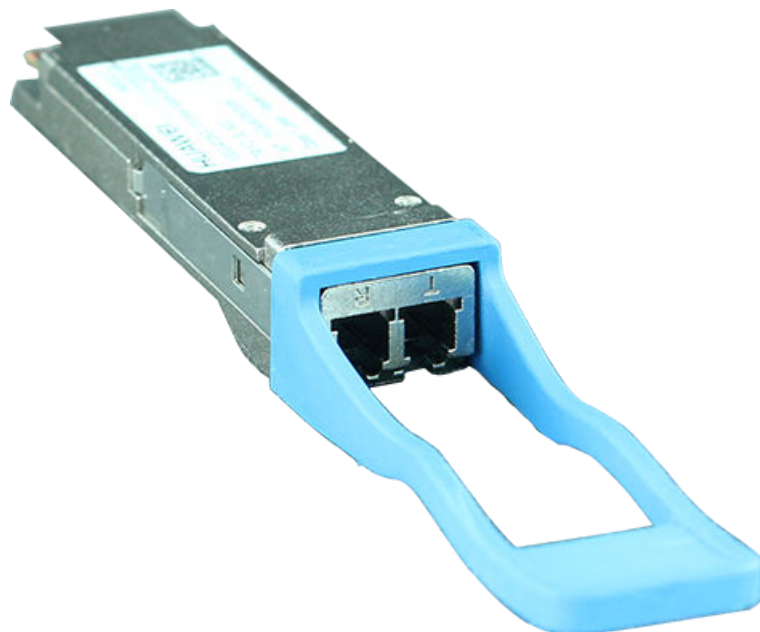
Figure 9-12 Appearance of a QSFP28 optical module (for LC optical fibers)
