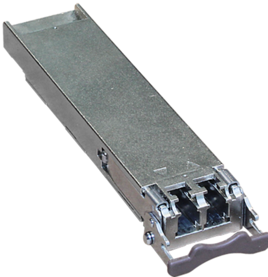
Figure 9-8 Appearance of an XFP optical module
